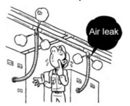
The pneumatic dampers were not opening the cooling enough to allow the air to condition this end of the building. So, by fixing the simple air leak I was able to reduce energy consumption significantly and save the facility \$180,000 in repairs. Again, with technology today there is a simple cost justified diagnostic solution.
