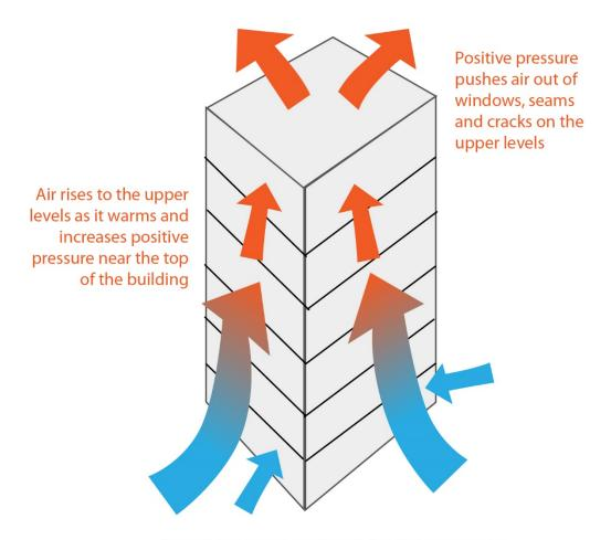
Negative pressure on lowels levels encourages infiltration of cold outdoor air through windows, doors, and openings
